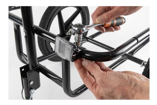
Attach the orange reflectors to the sides of the trailer.
